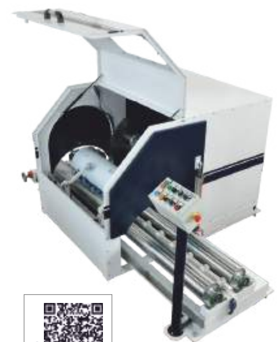
KAĞIT, LAMİNANT VE TESTERE KESİME UYGUN RULO FOLYOLARIN, RULODAN ÇÖZÜLMEDEN KESİMİ İÇİN DİZAYN EDİLMİŞTİR IT IS DESIGNED FOR CUTTING MATERIALS LIKE PAPER, LAMINATE AND ROLLED FOLDS WHICH ARE SUITABLE FOR SAWING WITHOUT UNWINDING FROM ROLL
